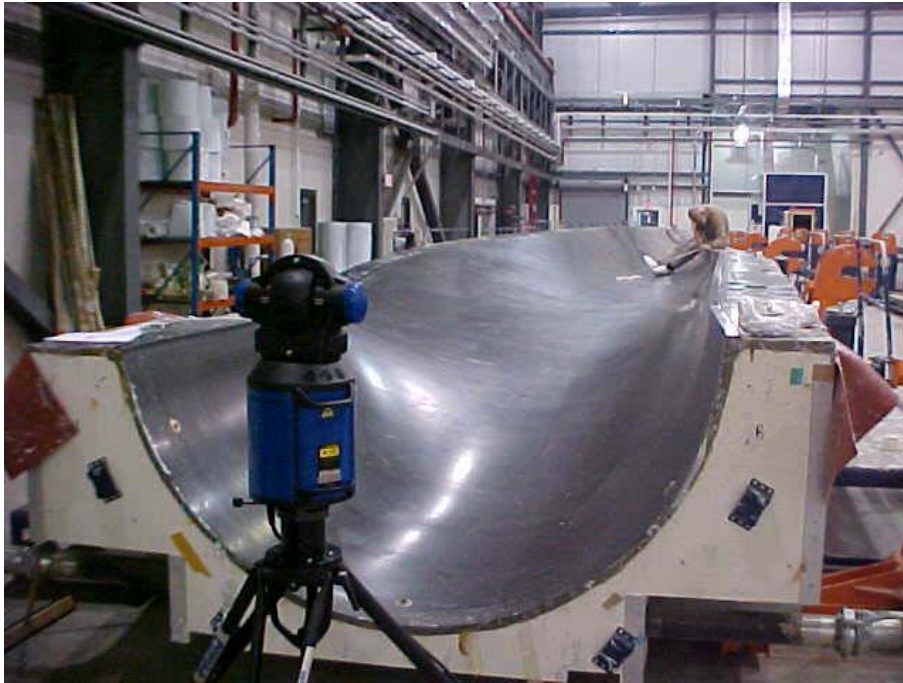
Figure 4: Photo showing the M-7 laser tracker preparing to measure a wind turbine blade mold
